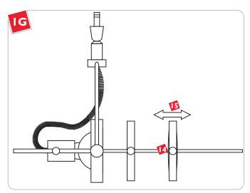
**NOTE:** The projected logo gets bigger and the intensity of the projected logo gets dimmer as the fixture is installed farther from the wall.
