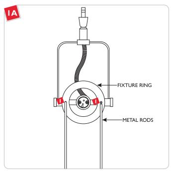
Screw the two metal rods completely into the threaded holes of the fixture ring.
