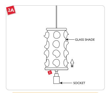
**NOTE:** To reduce the risk of a burn or electric shock during relamping, disconnect the power to the fixture.
