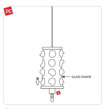
3 Lower the glass shade onto the socket assembly.
