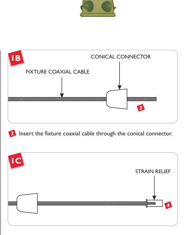
Insert the coaxial cable through the flared end of the strain relief.
