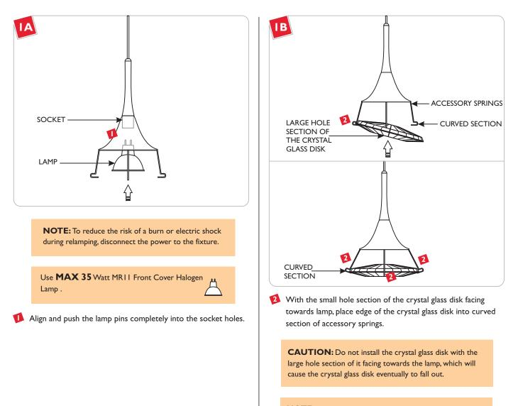
NOTE: The Crystal disk must be removed when relamping.
