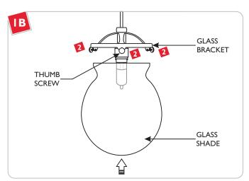
Place the glass shade completely into the glass bracket and tighten the three thumb screws to secure the glass shade in place.
