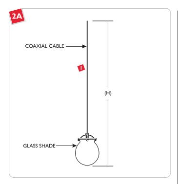
Cut the coaxial cable to the desired length with a sharp cutter. The overall fixture height (H) is measured from bottom of the glass shade to the end of the coaxial cable.
