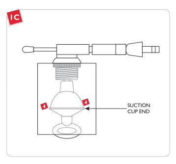
Remove the suction cup by picking on the ends.
