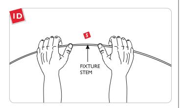
**5** Simply bend the fixture stem to the desired shape.
