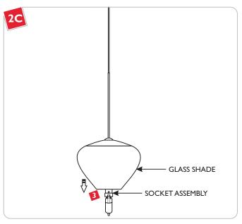
3 Lower the glass shade onto the socket assembly.
