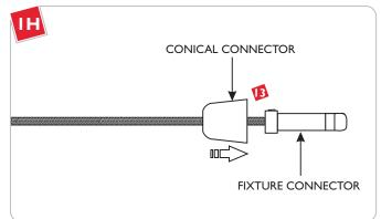
Slide the conical connector over the fixture connector. To install the fixture, refer to the instructions provided with the system.
