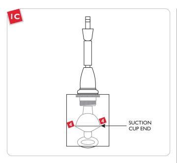
Remove the suction cup by picking on the ends.
