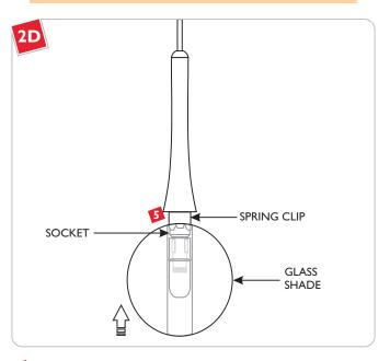
Replace and push the glass shade completely onto the spring clip.
