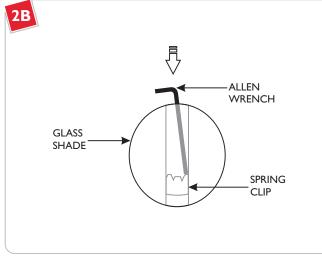
2 If the spring clip gets stuck in the glass shade, use the provided Allen wrench to remove it.
