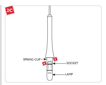
Place the spring clip back onto the socket make sure that the flat portion is against the socket cap.
