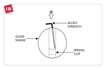
If the spring clip gets stuck in the glass shade, use the provided Allen wrench to remove it.
