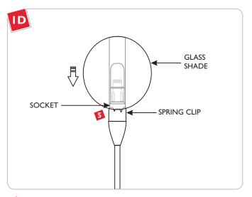
Replace and push the glass shade completely onto the spring clip.
