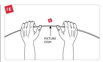
Simply bend the fixture stem to the desired shape.
