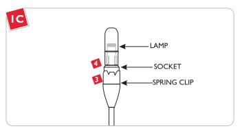
Place the spring clip back onto the socket make sure that the flat portion is against the socket cap.
