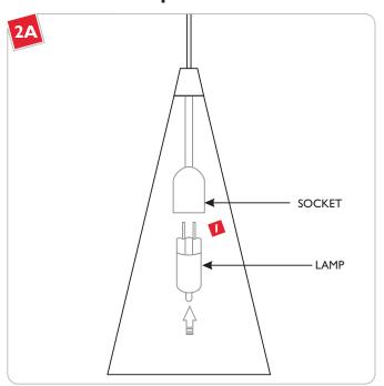
**NOTE:** To reduce the risk of a burn or electric shock during relamping, disconnect the power to the fixture.
