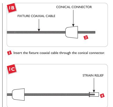
Insert the coaxial cable through the flared end of the strain relief.
