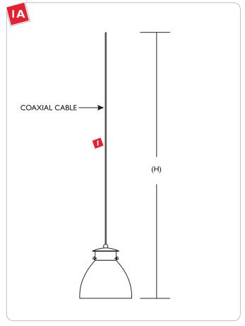
Cut the coaxial cable to the desired length with a sharp cutter. The overall fixture height (H) is measured from bottom of the glass shade to end of the coaxial cable.
