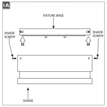
Unscrew and remove the three shade screws and separate the shade from the fixture base.
