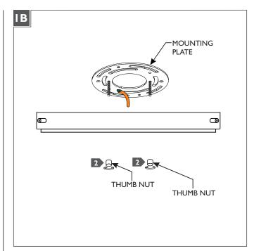
2 Separate the mounting plate from the fixture base by unscrewing the two thumb nuts.
