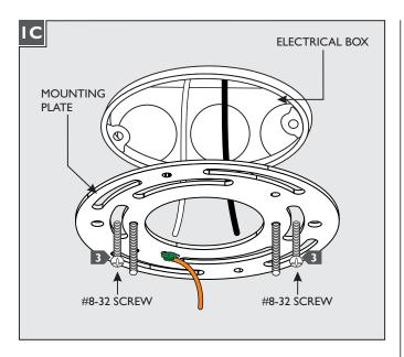
Mount the mounting plate to the electrical box with the two #8-32 screws.
