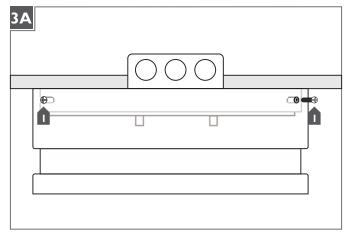
Align the screw holes in the shade with the fixture base and install the three shade screw by completely screwing them in.
