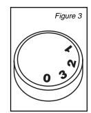
HIGH(3): For fast humidification of a large room. This setting will provide approximately 3 gallons of moisture output in a 24 hour period.\*
