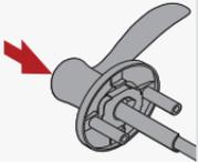
Push bolt to install exterior lever.
