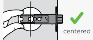
If the latch holes are NOT centered, adjust latch. See "Latch Adjustment" (step 1C).
