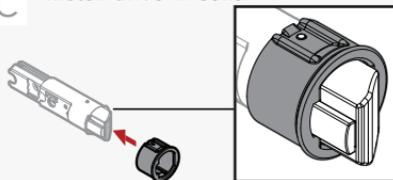
D Use hammer and wood block to tap in latch without damaging it.
