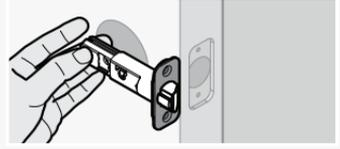
B If the latch holes are centered in the door hole, no adjustment is required. Proceed to step 2.
