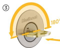
2. Fully insert new key and rotate 180°. Rotate back to starting position and remove key. **Your lock is now re-keyed!**
