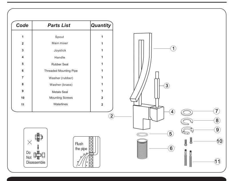
Do not disassemble the main body, as it has been installed & commissioned correctly & precisely before leaving the factory.
