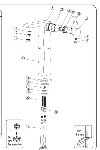
Do not disassemble the main body, as it has been installed & commissioned correctly & precisely before leaving the factory.
