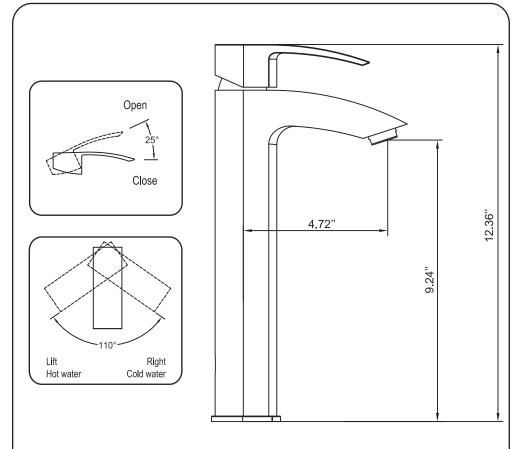
Make sure the installation holes are in the correct size. Install the lavatory and pop-up waste as shown in the drawing. Connect the main body and water supply pipe with water inlet pipe
