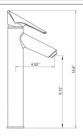
Make sure the installation holes are in the correct size. Install the lavatory and pop-up waste as shown in the drawing. Connect the main body and water supply pipe with water inlet pipe
