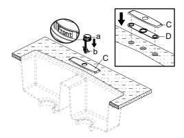
Place the escutcheon (C) and the gasket (D) on the sink. Insert the base (a) into the escutcheon (C). **NOTE:** "Front" on the base (a) must face the front of the sink. The two mounting plates (b) on the base (a) must be loose and movable during the installation of the base (a). If the sink is uneven, use silicone under the gasket (D).
