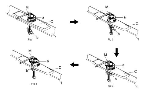
Press the base (a) and escutcheon (C) so that they can not move, then turn the screws with the provided hex wrench (M, HEX: 6.0mm) clockwise, as shown Fig 1. When the mounting plates (b) make contact with the sink (1), continue to turn the screw with the provided hex wrench (M, HEX: 6.0mm) clockwise, as shown Fig 2, until the base (a) is completely tightened and secured, as shown Fig.4.
