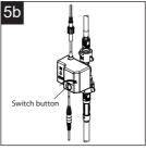
However, if you want to continue to use the faucet with the sensor feature, you need to tighten the switch button completely with a coin clockwise. At this time, you can use the faucet with the sensor feature.
