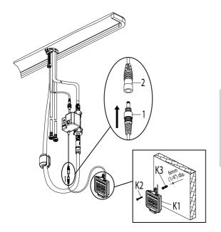
Drill a hole in the wall using a 6mm (1/4 in.) diameter drill bit. Install the battery pack (K1) using the molly anchor (K3) and screw (K2) provided. Insert the battery pack cable (1) into the control box connection (2).
