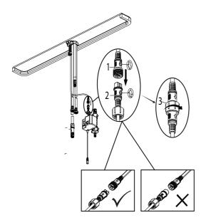
Install the data cable (1) to the control box connection (2). Ensure the arrows on the data cable and control box connection are aligned to one another to ensure proper installation. Ensure they are tightly connected by firmly pushing together. Secure the connection by hand tightening the nut (3) in a clockwise direction onto the threaded sensor cable.
