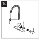
This indicates that the cartridge is damaged. Turn off the water supply, remove the handle and replace the cartridge (1).
