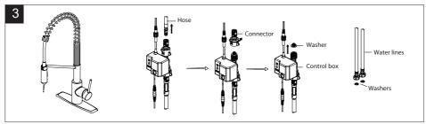
a. This could indicate that the washer in the control box is dirty or damaged. Remove the hose and unscrew the connector. Take out the washer from the control box. Clear the washer or replace the washer. Reassemble the connector and hose.
