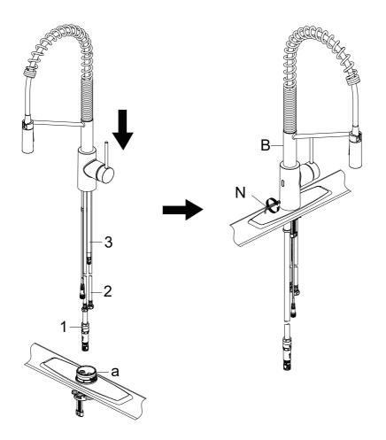
Insert the hose (1), supply lines (2) and quick connect hose (3) one by one through the hole of the base (a). Carefully insert the hoses into the base. Place the faucet assembly onto the base (a) as shown in the above figure. Secure the faucet assembly (B) by tightening the set screw with the provided hex wrench (N, Hex: 2.5 mm).
