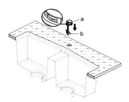
Shut off the water supply. Remove the old faucet. Clean the mounting surface. Check for the proper thickness of the sink. Insert the base (a) into the sink. If your model does have a escutcheon, skip to step 1 b.
