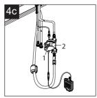
Check whether the switch button (1) is tight, if it is loose, tighten the switch button (1) completely with a coin clockwise. If the switch button (1) is tight, this indicates that the control box (2) is damaged. Call customer service to request a replacement control box. Replace the old control box with the new control box.
