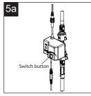
If you want to use the faucet without the sensor feature, you can loosen the switch button completely with a coin counterclockwise. At this time, you can use the sensor faucet just like a regular kitchen faucet.
