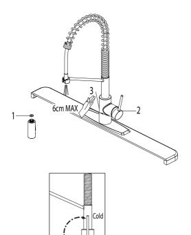
Flushing and checking for leaks: After the installation is complete, unscrew and remove the spray head in order to flush the line. Turn on the water supply and allow both hot and cold water to run for at least one minute each. This flushes away any debris that could cause damage to internal parts. Check for leaks. Reattach the spray head. Do not lose the gasket (1) in the hose.
