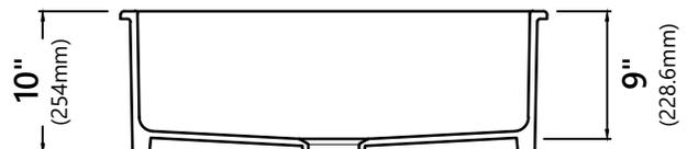
**NOTE:** Due to the typical  $\pm 3$ mm side wall variance in manufacturing, it is recommended that you design / modify the sink cabinet to match your clients individual sink(s) need.
