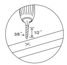
• Insert anchors into drilled holes and lightly tap with a hammer until flush.
