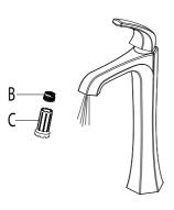
After installing the faucet, remove the aerator (B) with the included aerator key (C). Turn the water on for 30 seconds to remove any debris. Reassemble the aerator (B).
