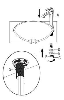
Place the faucet (A) through the hole in the countertop. Secure the faucet (A) to the countertop using the plastic washer (D), metal washer (E) and mounting nut (F) provided. Tighten screws (G).
