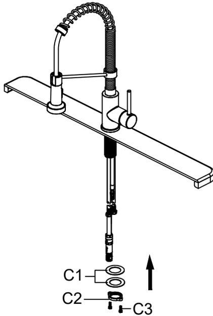
Install the rubber washer and metal washer (C1) onto the threaded mounting shank. Thread the nut (C2) onto the mounting shank. Lock the nut (C2) into position by tightening the screws (C3). Do not overtighten.
