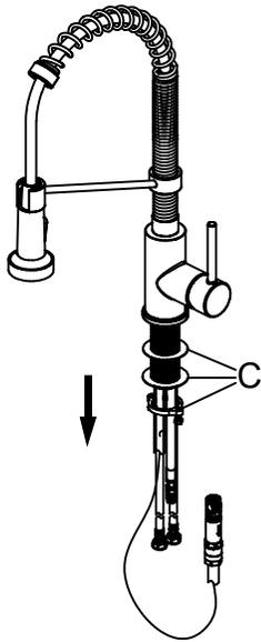
Shut off the water supply. Remove the old faucet. Clean the mounting surface. Remove mounting hardware (C) from faucet body (B).
