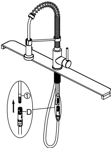
Push the quick connector (D) firmly upward and attach it to the receiving block (1). Pull down moderately to ensure the connection has been made.
