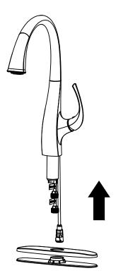
For three-hole installation: Deck plate, base plate (see below), and silicone sealant (optional) are required.
