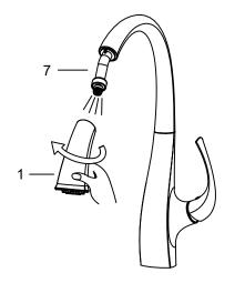
Remove spray head (1) from spray hose (7). Hold tip of spray hose (7). Turn faucet on and let the water run for 60 seconds to flush any debris.
