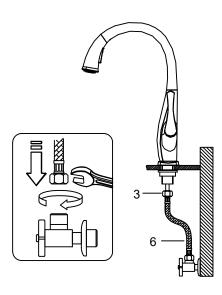
Connect waterlines (6) to hot and cold copper lines (3). Connect waterlines (6) to angle stops. Tighten both ends of waterlines with a wrench until snug. Turn on hot and cold angle stops and check for leaks.
