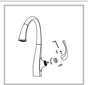
**Step 1:** Remove button located at the top of the handle. Loosen the set screw with a hex wrench. Remove the handle and unscrew cartridge cover by hand.
