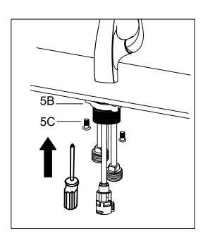
Adjust direction of faucet body (2) so that handle is on right side of faucet. Tighten mounting nut (5B) until snug. Tighten mounting screws (5C) to nut with a Phillips screwdriver until snug.
