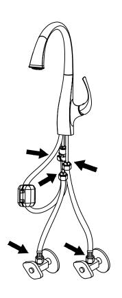
Check for leaks at the connections. Retighten if necessary.
