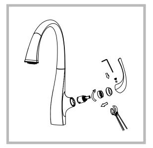
**Step 3:** Place the new cartridge in the handle seat. Secure the cartridge with the locking nut and assemble the handle.
