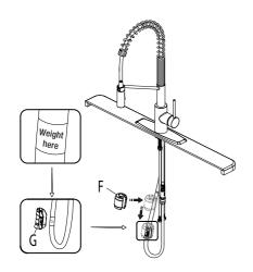
Install the weight clip (G) at the point of the hose marking "weight here". Insert the weight (F) onto the weight clip (G) by sliding it down onto the weight clip (G).
