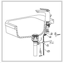
• Place one end of clip (n) on drain off pole (j). Insert drain off pole (j) through desired hole of extender rod (m). Place other end of clip (n) on drain off pole (j)
