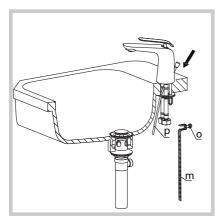
• Insert lift pole rod (p) through the hole in the back of the faucet body. Loosen thumb screw (o) and attach extender rod (m) to lift pole rod (p). Tighten thumb screw (o)
