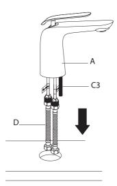
Remove faucet, mounting hardware, and waterlines from the box. Remove mounting nut (C4) from mounting screw (C3). Place faucet body (A) on a soft cloth, spout facing up. Secure hot & cold waterlines (D) at the base of the faucet (hand-tighten, then secure with <sup>1</sup>/<sub>4</sub> turn of adjustable wrench) A. Hot Side: Left B. Cold Side: Right Thread mounting screw (C3) into faucet base, flat head up, and tighten with a Phillips head screwdriver until snug
