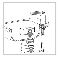
• Install drain (b), with rubber washer (c) attached, into the drain hole. Attach concave washer (d) with narrow end up, plastic washer (e), and mounting nut (f) to drain (b) from underneath countertop or sink. Secure tightly to sink with an adjustable wrench
