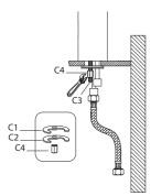
Install rubber U-washer (C1) and metal U-washer (C2) from underneath the countertop or sink. Attach mounting nut (C4) to mounting screw (C3) and tighten with adjustable wrench or 10mm wrench until snug
