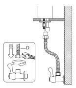
Thread hot & cold waterlines (D) onto angle stops and tighten with adjustable wrench until snug. Turn on angle stops and check for leaks (DO NOT TURN FAUCET ON)
