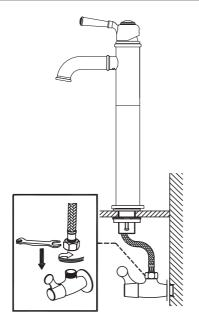
Connect flex water supply lines to angle stops and tighten with adjustable wrench. Turn on both hot and cold main valve
