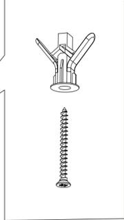
\*The provided drywall anchors should only be used with drywalls 1/2" thick or less.\*
