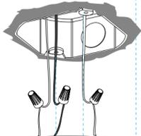
Feed the AC power cords from the LED drivers into the junction box through the hole as shown in the figure then connect them with the AC wires from the junction box. Secure the canopy to the junction box. Secure the canopy to the surround ceiling. Make sure the canopy is centered to the junction box and fully covering the junction box.
