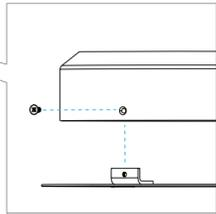
After wiring is completed, remove the hanging strings and secure the cover plate by fitting the two screws in from the sides.
