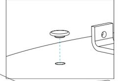
For Circular 3 model, cover the unused holes with the provided fillers.
