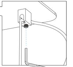
**2** Fit the cable through the cable holder and tighten using the provided hex key. Lower each pendant to desired height.
