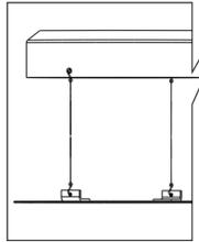
Use the provided strings to hang the cover plate from the canopy during installation
