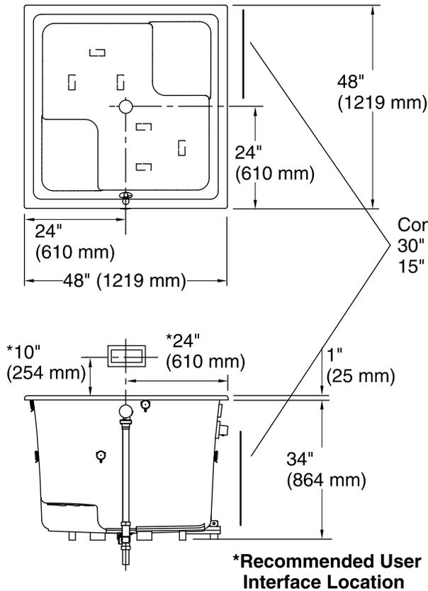
No change in measurements if connected with drain illustrated. (K-8150)
