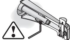
Overtightening may damage copper pipes!
