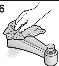
Remove the excess sealant.
