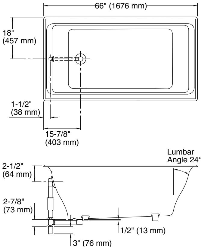
No change in measurements if connected with drain illustrated. (K-7147-AF)
