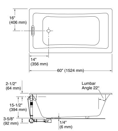
No change in measurements if connected with drain illustrated. (K-23856-NA)
