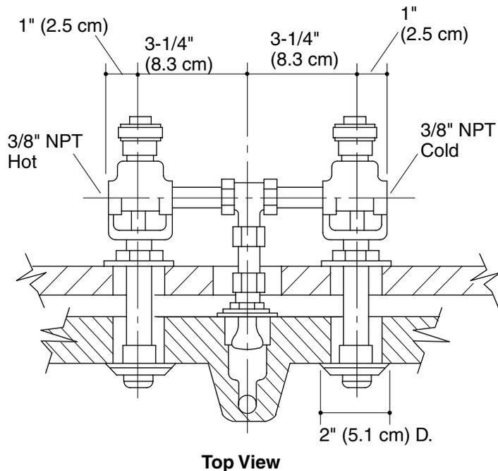
**Note:** Supply fitting required furnished for wall not to exceed 1" (2.5 cm) thick. For thicker wall add 1" (2.5 cm) to supply measurement [3" (7.6 cm)] for every inch or
