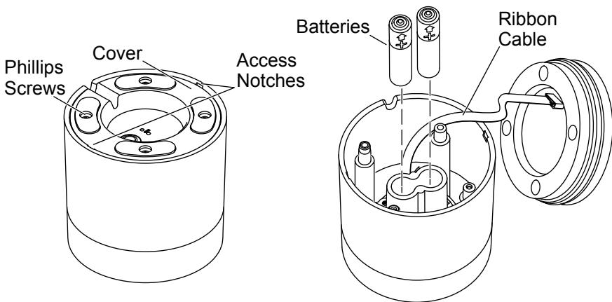
**NOTE:** If the remote control no longer charges or needs to be recharged too often, the batteries can be replaced.
