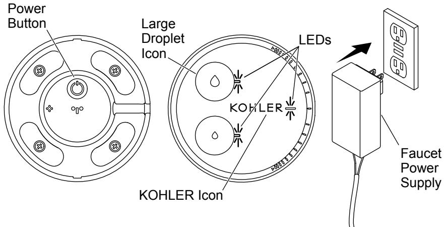
**NOTE:** Connect the charger if pairing a new remote control.
