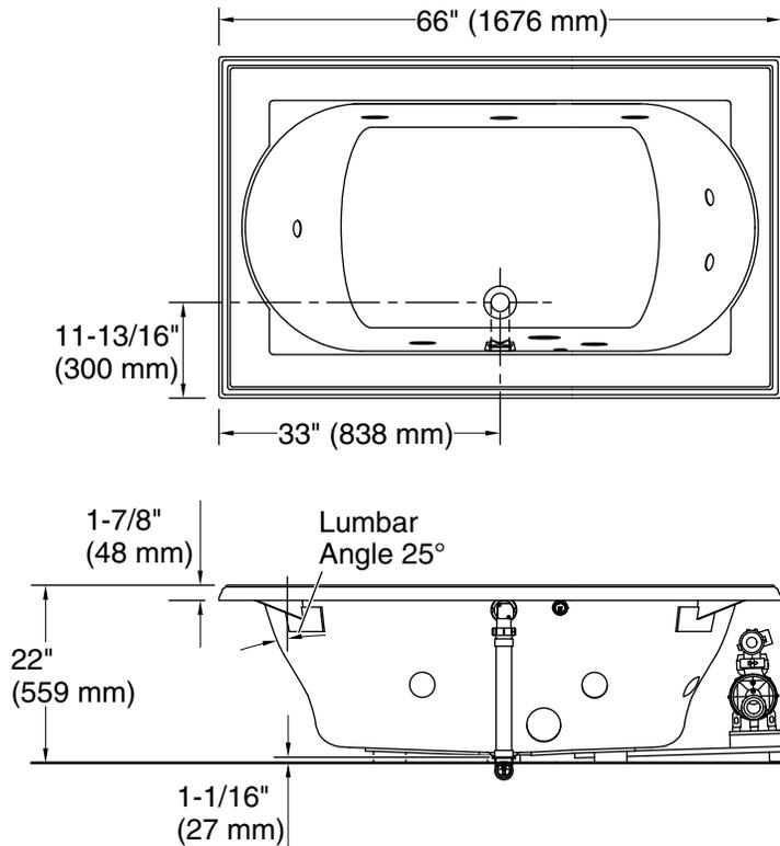
No change in measurements if connected with drain illustrated. (K-7161-AF)
