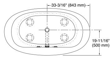
No change in measurements if connected with drain illustrated. (K-T37391-CP)
