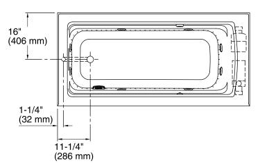
No change in measurements if connected with drain illustrated. (K-7271 or K-7272)
