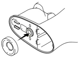
**4** Carefully lower the toilet onto the flange, holes aligned with the depth gauges.
