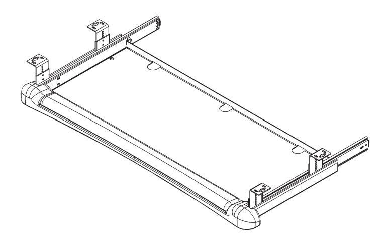
Note: Brackets mount in outboard position under work surface for application widths 29" or greater, and in the inboard position for widths less than 26.7"
