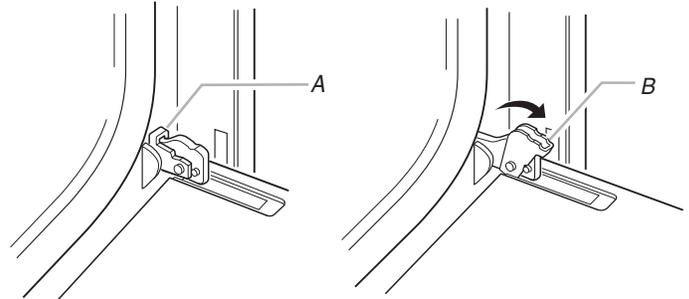
3. Grasp the edges of the oven door with both hands and close the oven door until it will no longer close. Lift and pull oven door toward you and remove. Set the oven door(s) aside on a covered work surface.
