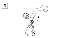
6. Wrap Teflon tape around all the threads on shower arm and hand tighten the shower head clockwise.
