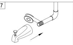
7. Apply pipe compound to tub spout nipple and attach spout to nipple. Hand tighten.
