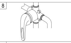
8. Turn on water supply and check connections for leaks. Place handle on valve stem and flush lines by running hot and cold water uninterrupted for one minute.
