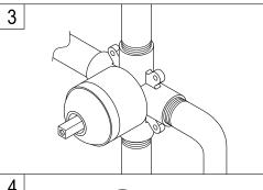
3. Connect water supply lines to valve. (Hot water to left and cold water to right side of valve.) Use compound or tape on all threaded connections. Connect valves to spout.
