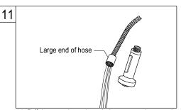
11. Pull the spray hose through the spout and secure the end into the drain, or have a secure party hold the spray hose, and turn on the faucet and flush for one minute. Attach spray head to the large end of the stainless steel hose. Insert spray head onto faucet body.
