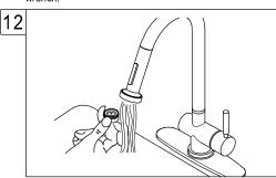
12. Remove the aerator before turning on your new faucet for the first time, let hot and cold water run for at least 1 minute, replace aerator this will prevent debris in the line from clogging the aerator.
