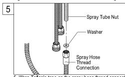
5. Wrap Teflon's tape on the spray hose thread connection and connect the spray hose to spray tape and secure with spray tube nut. Tighten with wrench carefully.
