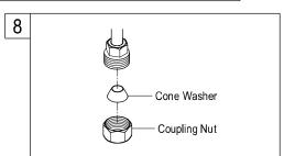
8. if you have 3/8" supply tubes, use the 3/8" friction ring that is in the parts bag. If you have 1/2" supply tubes, use the 1/2" friction ring that is in the parts bag. Place the friction ring and cone washer into the coupling nut as shown in the above illustration, and then connect. HAND TIGHTEN ONLY, AND BE CAREFUL NOT TO OVER TIGHTEN. One full wrap of teflon tape is required on all threaded connections. Caution: Do not let the tubing revolve or bend when tightening.
