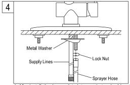
4. After installation is completed, turn on hot and cold water supply valves. (Be sure the faucet is in off position before turning on the supply valves) Then check for any leaks, especially at hook-ups to supply lines. Tightening nuts slightly will stop and minor leaks.
