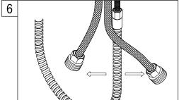
6. Insert the hose through the guide and attach to the fitting on the bottom of the faucet.
