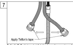
7. Apply Teflon's tape to inlet shanks and connect supply lines.
