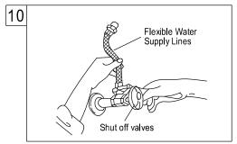
10. Connect the water supply lines. Before connecting the supply lines, apply pipe joint compound to the threads on the inlet shanks and shut off valves with an adjustable wrench.
