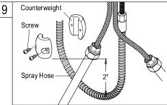
9. Install counterweight set on the spray hose. Adjust the counterweight at least 2" higher then the bottom line as illustrated. Fix with screws tightly.
