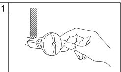
1. Turn off water supply valves under the sink. Cover the sink drain so that no small parts are lost down it. Remove your old faucet. Caution: Do not damage your old water supply lines. Clean the surface of the sink in preparation for installing the new faucet.
