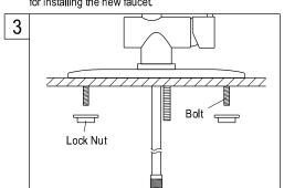
3. Fit faucet onto the sink. Secure faucet by threading and tightening wing-nuts onto studs.
