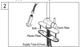
Place deck plate in proper position, put hose and supply tubes through center hole of deck plate. Install hold down bolts onto brass deck plate by sliding stud into the notched receptacle on the base plate. Place plastic plate under the deck plate smooth side down.
