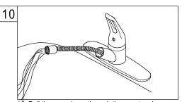
10. Pull the spray hose through the spout and secure the end into the drain, or have a secure party hold the spray hose, and turn on the faucet and flush for one minute.
