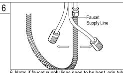
6. Note: if faucet supply lines need to be bent, grip tube at point of bend with right hand, firmly and slowly pull tube into position using rounded bend with left hand. Extreme care must be exercised. Follow instructions exactly. Kinked tubes will void warranty.
