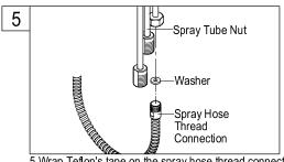
5. Wrap Teflon's tape on the spray hose thread connection and connect the spray hose to spray tape and secure with spray tube nut. Tighten with wrench carefully.
