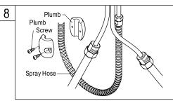
8.Install counterweight on the spray hose and adjust the counterweight at least 2"higher than the bottom line as illustrated. Fix with screws tightly.
