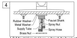
4. Pull the stainless steel hose up through the faucet until the attachment nut is up against the bottom of the faucet shank. Install rubber washer and metal washer on the faucet shank and secure with brass nut, tighten wrench tight. (Have patience when slipping the brass nut past the water tube connections, it will fit past them.)
