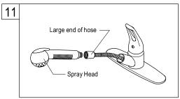
11. Attach spray head to the large end of the stainless steel hose. Insert spray head onto faucet body.
