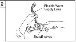
9. After completed the installation, be sure the faucet is in off position before turning on the hot and cold supply valves to check for leaks, especially at hook ups to supply lines. Tightening nits slightly will stop any minor leaks.
