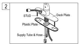
2. Place deck plate in proper position, put hose and supply tubes through center hole of deck plate. Install hold down studs onto brass deck plate by sliding stud into the notched receptacle on the base plate. Place plastic plate under the deck plate smooth side down.
