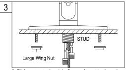
3. Fit faucet onto the sink. Secure faucet by threading and tightening wing-nuts onto studs.
