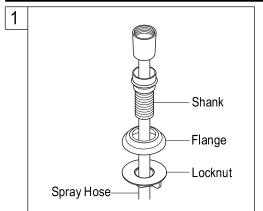
1. For model is with spray head and hose. Place the spray guide through the fourth hold in the sink, screw the locknut onto the shank and tighten firmly.
