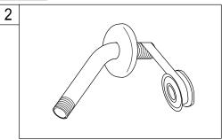
2. Wrap threads on one end of shower rod male nipple with 4 to 6 wraps of teflon.
