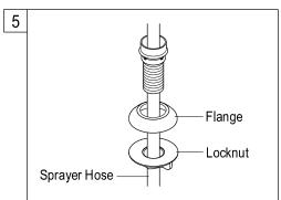
5. For model is with spray head and hose. Place the spray guide through the fourth hold in the sink, screw the locknut onto the shank and tighten firmly.
