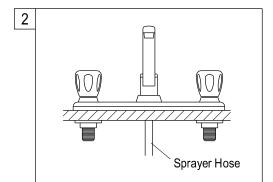
Set the faucet in place, insert the inlet shanks through the sink holes, and press down.
