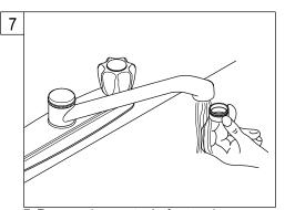
7. Remove the aerator before turning on your new faucet for the first time. This is to prevent any deposits from clogging your aerator. Allow both hot and cold water to run for one minute. Replace aerator.
