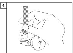
4. Turn on water supply valves and check for leaks, especially at hook-ups to supply lines.
