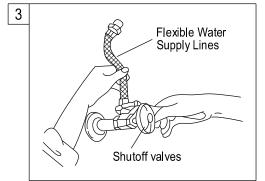
Connect the water supply lines. Before connecting the supply lines, apply pipe joint compound to the threads on the inlet shanks and shut off valves.
