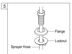
5. For model is with spray head and hose. Place the spray guide through the fourth hold in the sink, screw the locknut onto the shank and tighten firmly.
