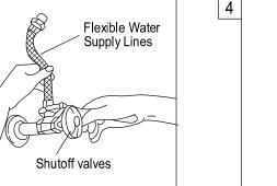
3. Connect the water supply lines. Before connecting the supply lines, apply pipe joint compound to the threads on the inlet shanks and shut off valves.
